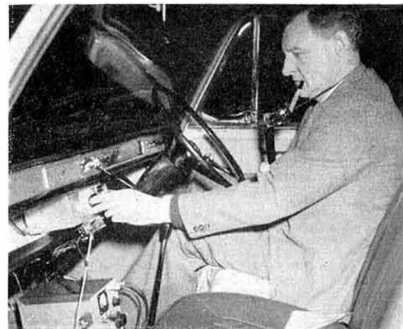
This photograph of G2CLN/M operating his 160m mobile rig was taken on 12 March at an exhibition on Amateur Radio organized by the Bromsgrove Amateur Radio Club. The apparatus is home-constructed, comprising a transistorized receiver and a valve transmitter. A loaded whip is mounted on the rear bumper of the Austin 1100. (Photo by courtesy of the Bromsgrove Messenger)
