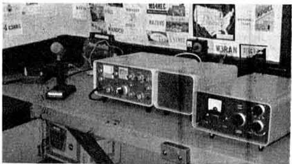
Layout of h.f. station: left to right, Shure microphone, KW2000A transceiver and the Green LA600 linear amplifier.
