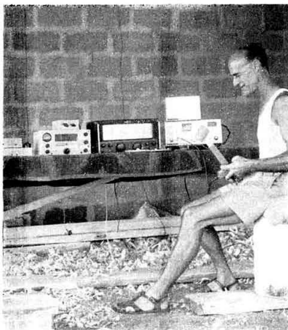
VQ8BFA operating ashore on Agalega Island. The equipment is a home-built 20 watt c.w./a.m. transmitter, an Eddystone 750 receiver, and an NCX-3 transceiver.
